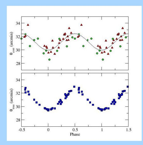
Top: actual measures of the Moon's angular diameter, using a simple sighting device.
