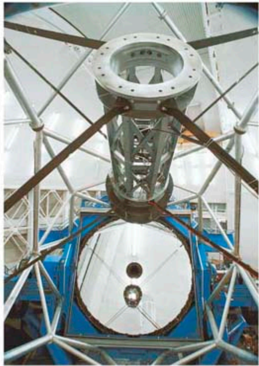
b The Gemini North telescope, located on the summit of Mauna Kea, Hawaii, is a reflecting telescope with the Cassegrain design. The primary mirror, visible at the bottom of the large lattice tube, is 8 meters in diameter. The secondary mirror, located in the smaller central lattice, reflects light back down through the hole visible in the center of the primary mirror.
