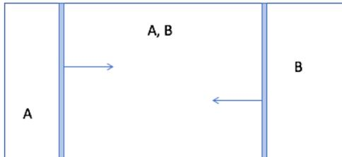
equal numbers. Semi-permeable pistons are slowly moved from the far right and left ends of the cylinder as shown until they meet in the middle, dividing the cylinder into two equal halves. The pistons are semi-permeable: the one on the right allows B atoms to pass freely, but A atoms cannot go through, while on the left is the opposite situation with only A passing freely. (Membranes sometimes used to desalinate
