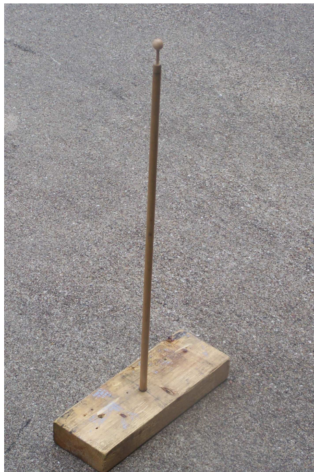
Figure 1. A gnomon, consisting of a vertical stick with a small sphere at the top. If we mark the center of the elliptical shadow of the sphere, we can get an accurate shadow length that corresponds to the elevation angle of the center of the Sun above the horizon.
