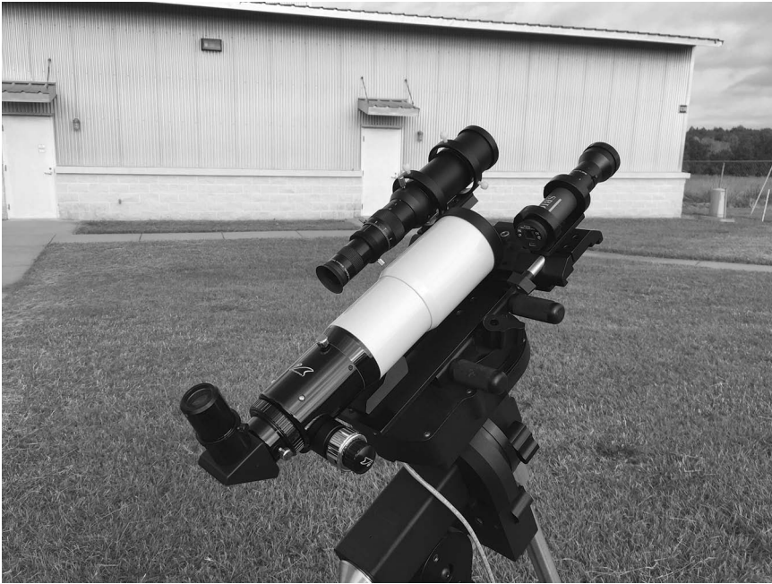
Figure 12.1 The SBIG camera is the small tube on the upper right. The other two telescopes are just finder scopes. Photo courtesy of Don Carona.
