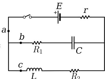
What is the current at the points  $\ a$  \_\_\_\_\_,  $\ b$  \_\_\_\_\_, and  $\ c$  \_\_\_\_\_ immediately after  $\ ^t_0$  ?
