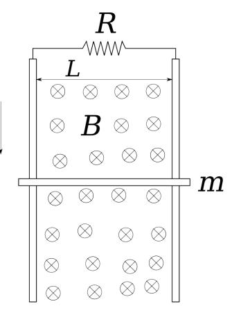
What is the direction of electric current induced by the motion?(show on the figure)
