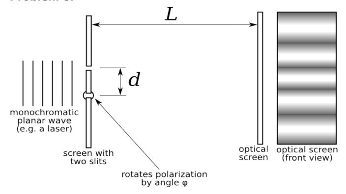
In the two slit experiment the polarization of the light from one of the slits is at angle  $\phi$ =30° to the polarization of the light from the other slit. The light from both slits have equal intensities. The distance between the slits is d=0.46mm . The screen is at distance L=2.54m . The adjacent bright fringes are separated by 2.82mm.
