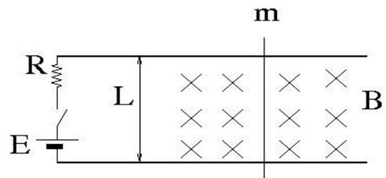
What is the current through the bar right after the switch is closed?\_\_\_\_\_
