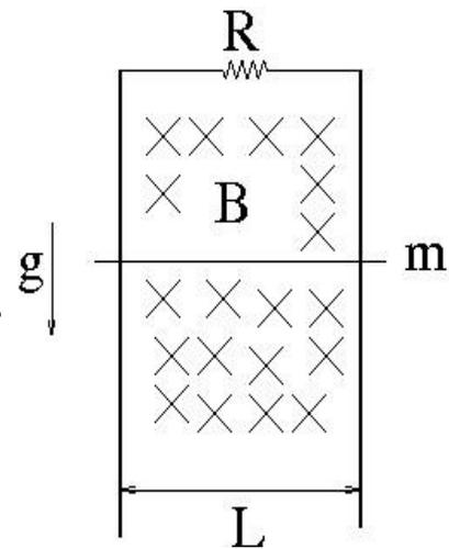
What is the direction of electric current induced by the motion?(show on the figure)
