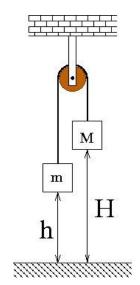
What is the velocity of the brick M right before it hits the floor?\_\_\_\_\_
